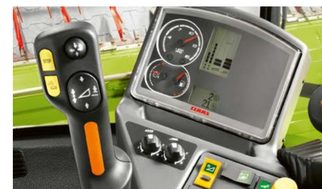
AUTO CONTOUR is activated simply by pressing the height adjustment button on the multifunction control lever.
