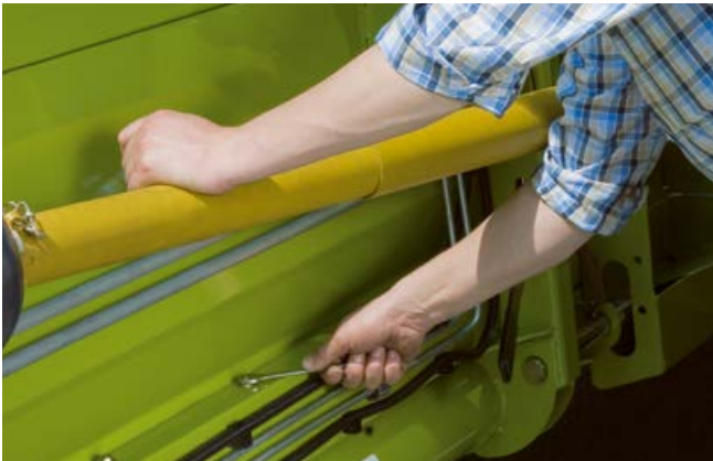
Stripper bars adjustable from outside (C 490, C 430, C 370).
