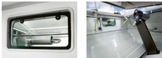
Large grain tank capacity AVERO 240: 5,600 l AVERO 160: 4,200 l
