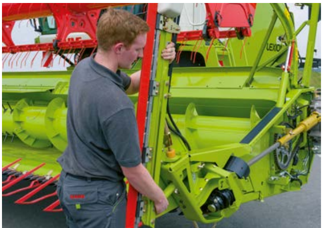
Rapeseed knives fitted by means of quick-release mounting system.
