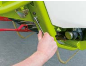
Easy adjustment of divider height using the panel key.
