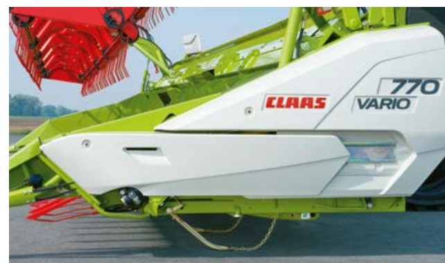
Sensor bands immediately behind the knife bar detect the position of the cutterbar.
