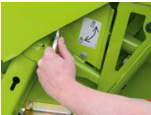
The crop dividers can be secured without tools thanks to the quick-release mounting system.
