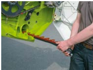
Replacement knife bar stored underneath the cutterbar.
