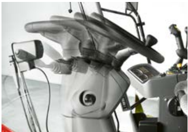
The steering column is adjustable three ways.
