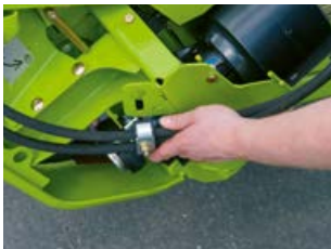
Easy connection of the hydraulic hoses for the rapeseed knife drive.
