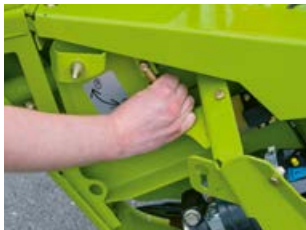
The crop dividers and rapeseed knives can be secured without tools thanks to the quick-release mounting system.
